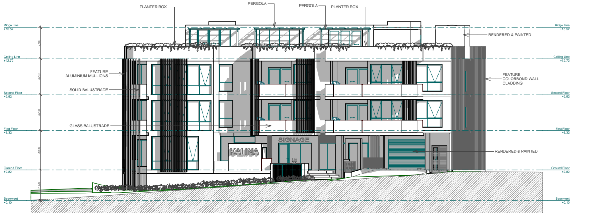
South West Elevation 1:200
